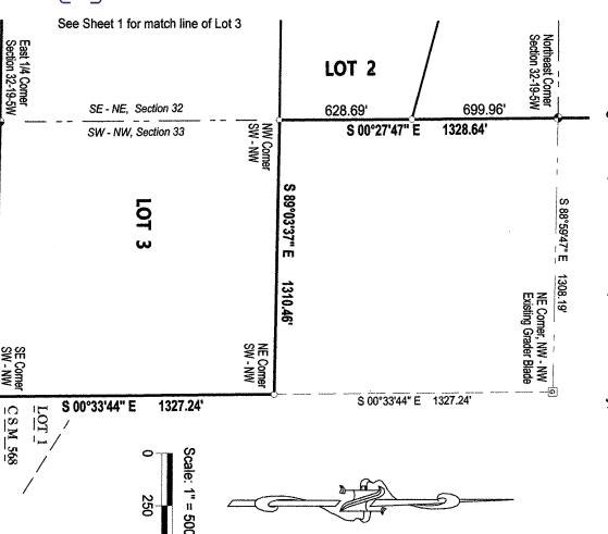
Northwest corner, a downed fence wire going North-South was right on, and at the Northeast corner an thin walled 1/2" iron pipe and steel fence post were found. No points on line from CSM 568 were located. Evidence noted lying 18-20' South of the North line of the SW - NW, Section 33: Fence post and partial fence headed East from the
